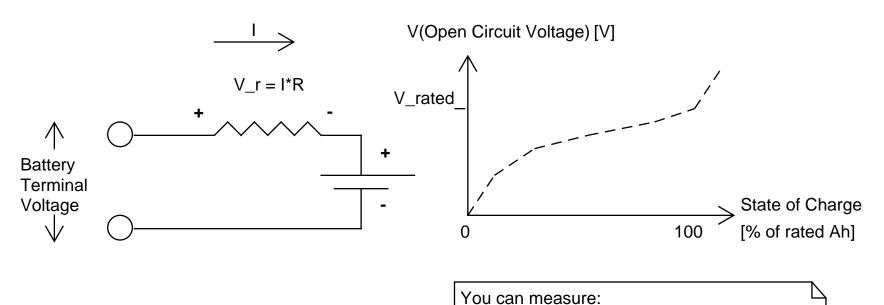
Battery Terminal Voltage = V\_r + V\_ocv Battery Terminal Voltage = I\*R + V\_ocv
