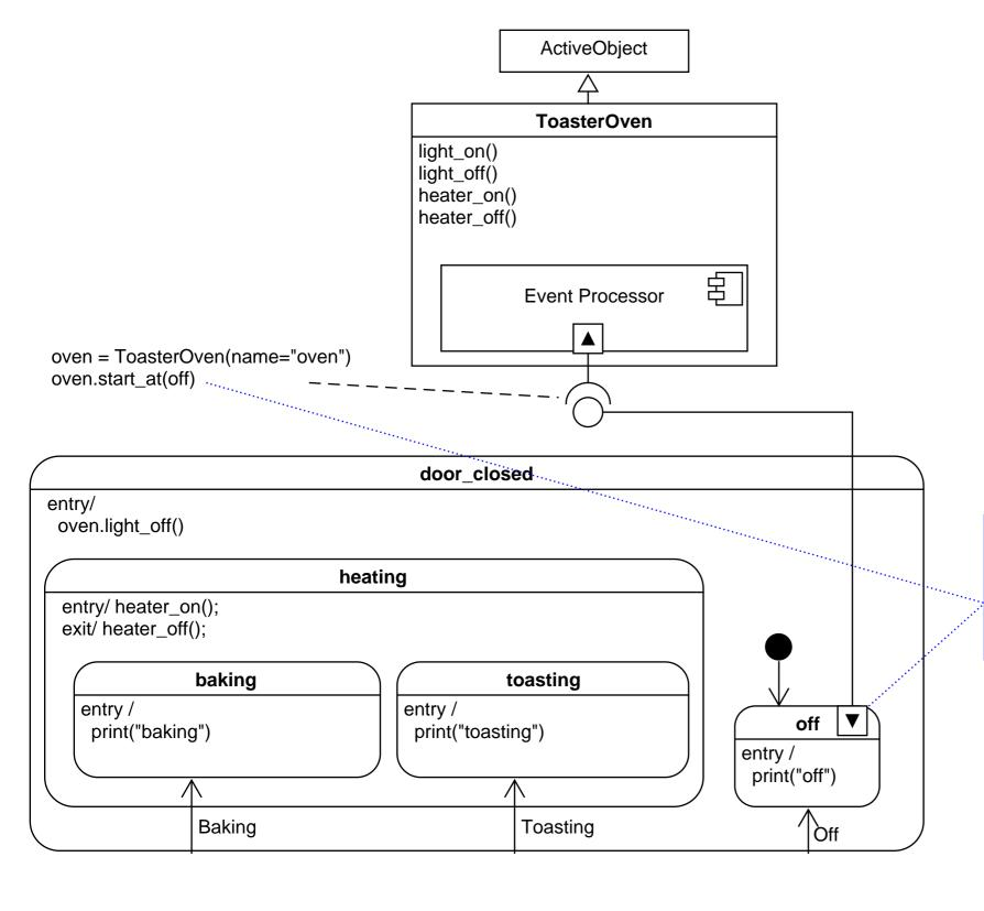
The attachment point in the drawing is connected to the off state
